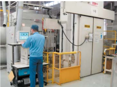
Automatic conditioning and electrical testing device
