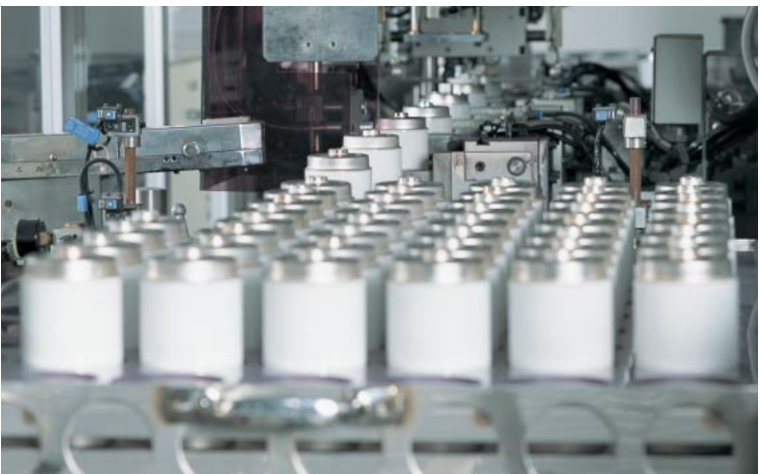
Fitting of a guide, measurement of vacuum degree and bellows force are carried out automatically
