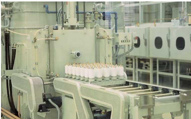
Continuous vacuum furnace
